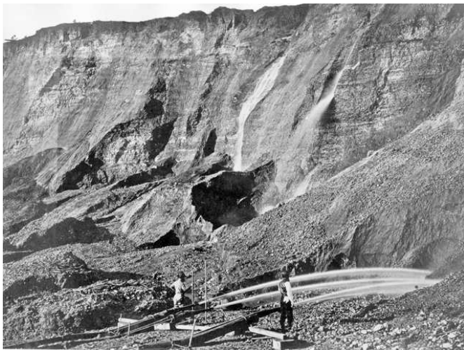
Figure C-4-1. Hydraulic Mining Water Cannon
